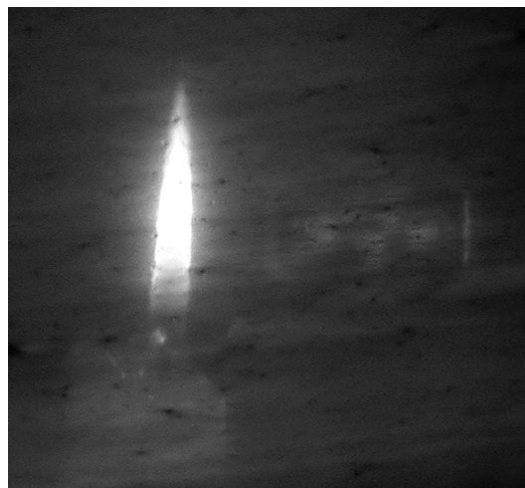
Fig. 10: Candle and white LED lamp with black polyethylene foil in IR mode.
