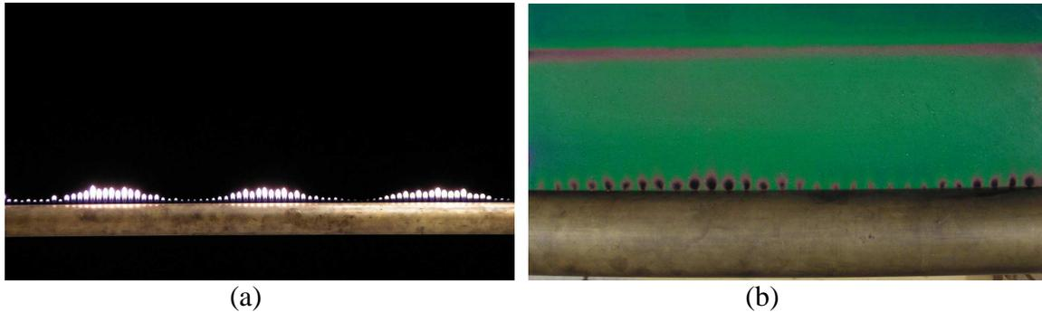
*Figure 7 The distribution of nodes and antinodes in a Rubens' tube visualized by flames (a) and TSF (b).*
