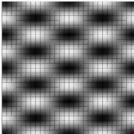
*Figure 6 Power density distribution of an electric field in the cavity of a MW oven. Theoretical calculation for (2,4,1) mode. The distance of neighbouring gridlines is 1 cm.*
