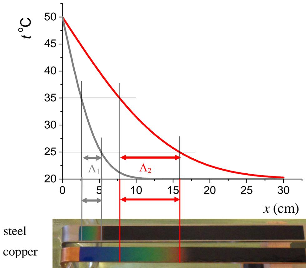
Figure 3 The theoretical temperature distribution in copper (red) and steel (grey) rods compared with the distribution experimentally detected using TSF.
