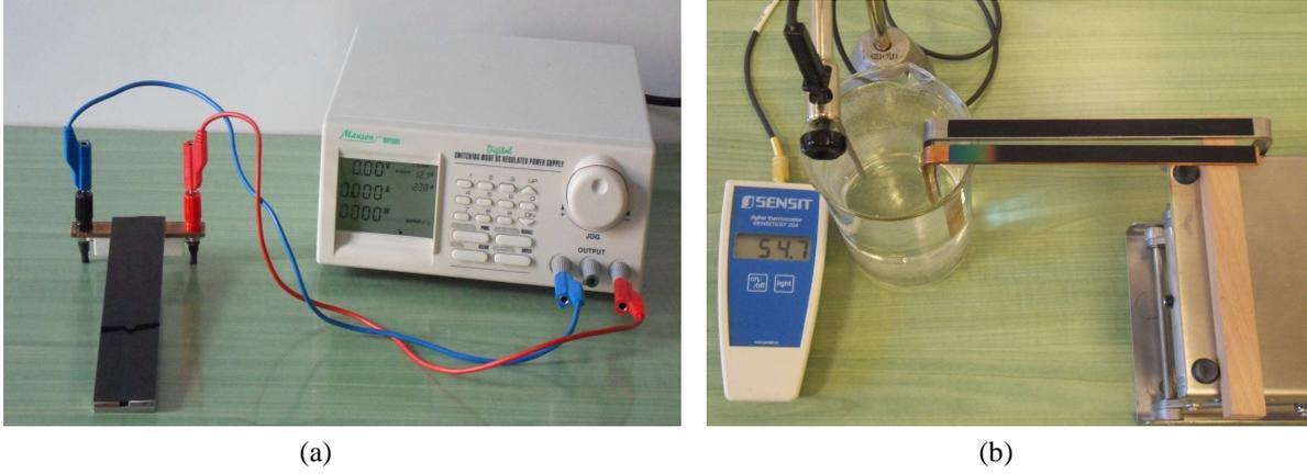
Figure 2 Two metal rods heated with a power resistor (a) or hot water (b).
